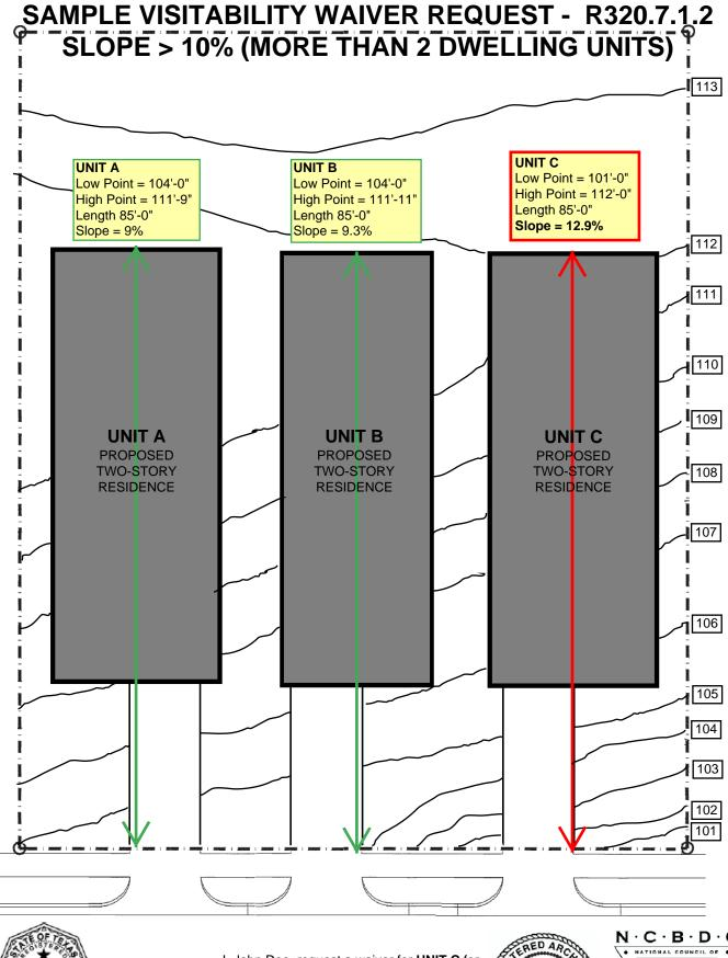
SURVEY DATE: 07-01-2015 SCALE: 1" = 40' I, John Doe, request a waiver for <u>UNIT C</u> for the exterior visitable route in compliance with R320.7.1.2 due to slope of lot between highest point at rear of structure and lowest point at property line exceeding 10%.
